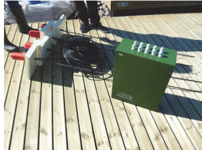
Electrodes for electrokinetic treatment of sediment
