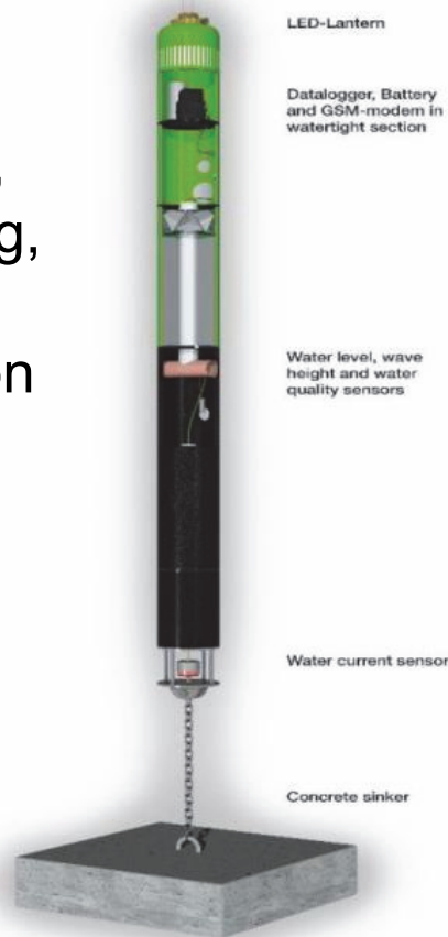
Schematic diagram of the SmartBuoy concept
