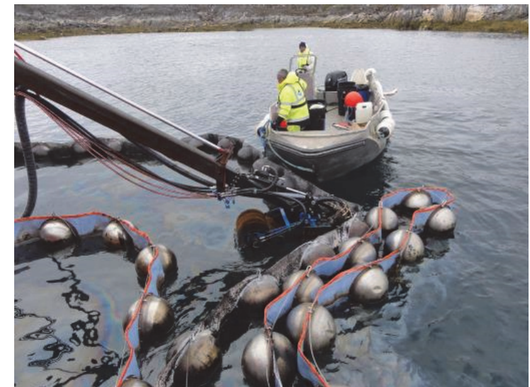
Collecting burning residue with Bucket Skimmer, Greenland
