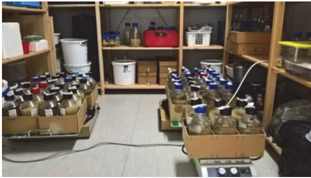
Biodegradation tests at 4 °C
