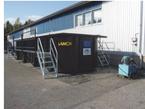
Test tank in Porvoo for testing oil collection
